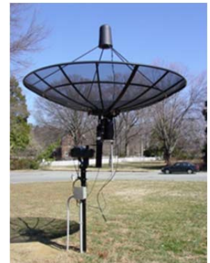
10-ft Alt/Az Mounted Satellite Dish at Randolph-Macon College
