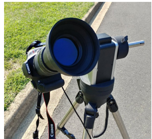
My Setup: iOptron ProCube Mount, Canon 300mm Lens, 1000 Oaks Optical Solar Filter, Canon Rebel t5. Credit: Tom Watson
