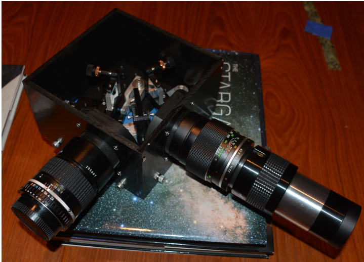
Bart's Common Path Interferometer. Credit: Bart Billard
