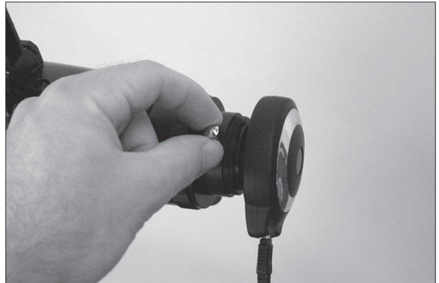
**Figure 2.** The SSSSI-III fits into 1.25" focusers, just like a standard 1.25" eyepiece.
