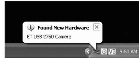
**Figure 4.** When initially connecting the SSSSI-III to a computer, a **Found New Hardware** notification will appear and automatically install the camera to your computer.
