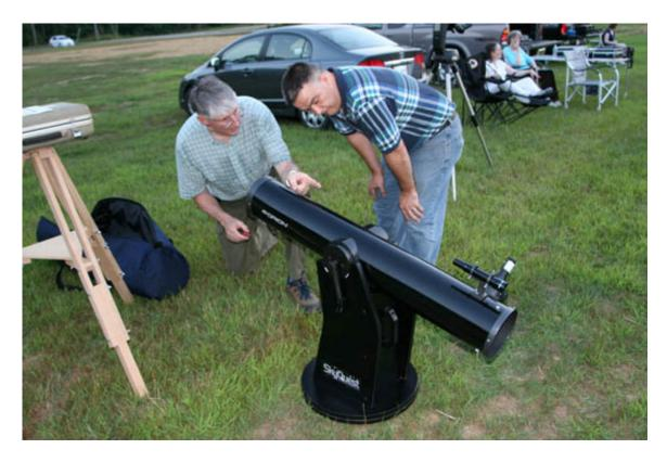
Joe and Ranny using a Laser Collimator to align the primary mirror
