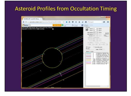
This is from the online results page for a recent observation with 11 participants. Each station's result shown as a star trail parallel to the predicted centerline of the predicted shadow path. They are adjusted so they appear as though the stations were all lined up perpendicular to the path, resulting in the blank area showing the apparent shape of the shadow:
