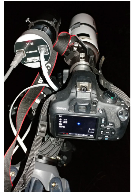
Telescope connected to auto guider Credit: Tom Watson
