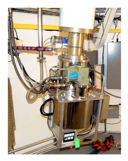
VLA Detector Vacuum Manifold with flange o-ring seal, manual vent valve, solenoid roughing valve, thermocouple vacuum gauge, and KF flange connection to roughing line.
